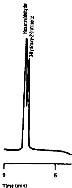
Fig. 6. Separation of dansyl-hydrazone of hexanal and 3-hydroxy-2-butanone. Mobile phase, diisopropyl ether; 0.5% of BOP on Zipax ® ; flow-rate, 1 ml per 66 sec.
